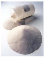
Firing sand FRSAND Fine sand for porcelain firing; allows porcelain to shrink without warping. Re-usable; no pre-firing required. Wt.: 3lbs. (1.35kg). Warning: Wear protective mask when using.
